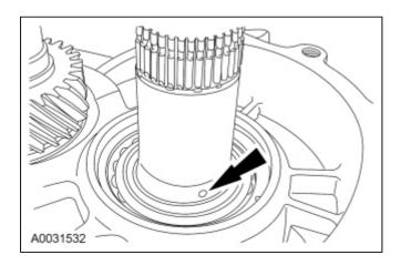
36. **NOTE:** The thrust washer is positioned with the flat surface facing upward towards 5th gear.
