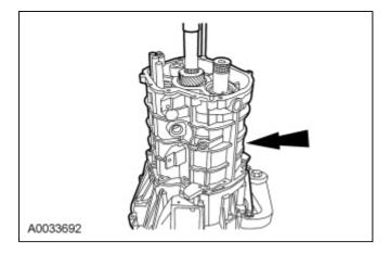
17. **NOTE:** Rotate the countershaft to seat the bearings.
