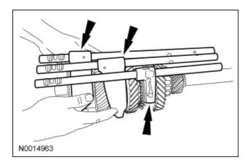
12. NOTE: The notches on the shift rail should be pointing upward.
