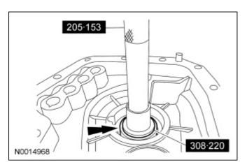
24. Using the recorded end play measurements, select and install the appropriate shims to achieve the correct end play.
