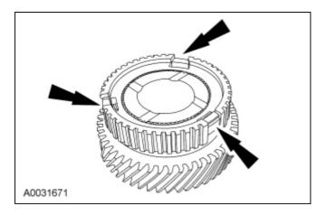
38. **NOTE:** Align the pockets in the blocking ring with the struts in the synchronizer.
