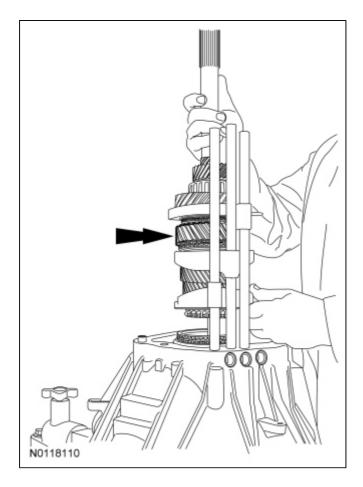
28. Using a jack and a block of wood, lift the mainshaft 13 mm (0.511 in) upward, then tilt the countershaft inward and install the countershaft.
