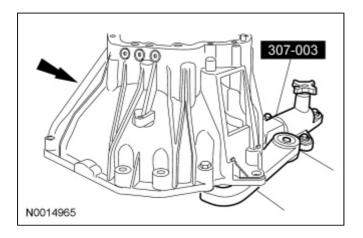
3. **NOTE:** If a new rear output shaft bearing was installed or a new rear countershaft bearing is being used, install new bearing cups.
