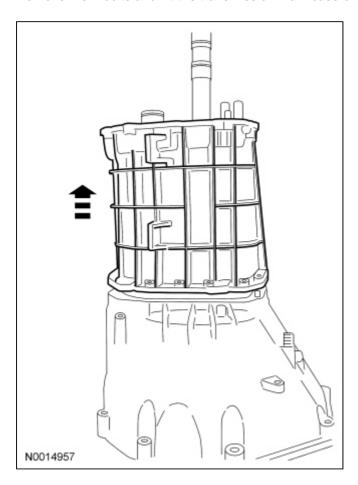
19. Using a jack and a block of wood, lift the mainshaft 13 mm (0.511 in) upward, then tilt the countershaft outward and remove the countershaft.
