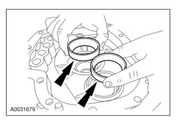
23. Using the Input Shaft Oil Seal Installer and Handle, install the new input shaft seal.
