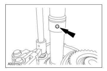
49. **NOTE:** The OSS sensor tone wheel is brittle. Gently tap the tone wheel into position.
