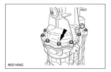
56. **NOTE:** If a new rear output shaft bearing was installed, install a new bearing cup.
