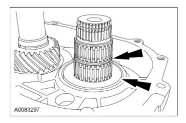
37. Place the 5th gear synchronizer blocking ring and the synchronizer hub on the countershaft 5th gear. Install the synchronizer springs and inserts.
