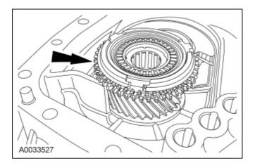
27. **NOTE:** The notches on the shift rail should be pointing upward.
