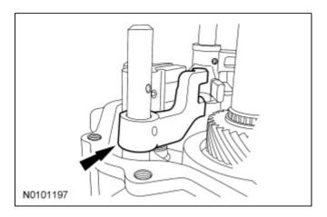
42. **NOTE:** Lubricate the shift rail with transmission fluid. Using a plastic hammer, alternately tap the shift fork and the synchronizer cone into position.
